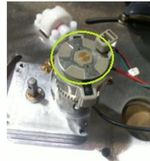
Sweep Motor (Timing Disc highlighted in green). Visible through the
