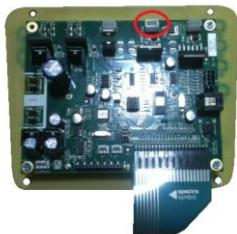
Control Panel J14 Elevation plug.
