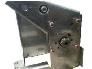
Unscrewing Elevation Motor Screws.
