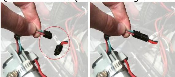
**Step 7.)** Reconnect the Elevation Motor wire into the J14 Elevation tab on the control panel.
