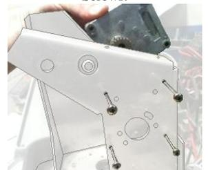
Removing Elevation motor.
