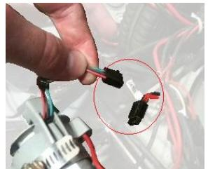
Elevation Quick disconnect disconnected.
