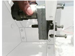
The Elevation Motor being held into place.
