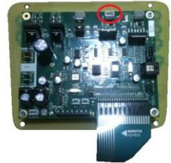
Control Panel J14 Elevation plug.
