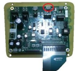
Control Panel J14 Elevation plug.
