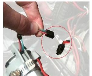
Elevation Quick disconnect disconnected.
