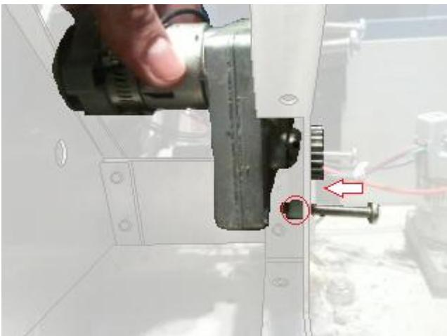
**Step 5.)** Hold the new motor into position with one hand, (Make sure the motor is Top is at its highest elevated point), and proceed to fasten the 4 screws down.
