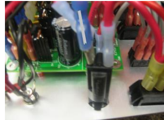
f. Battery Positive wire (shown in light grey)
