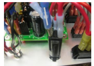
f. Battery Positive wire (shown in light grey)
