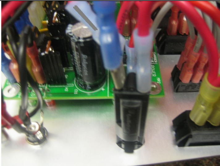
The positive XLR wire (shown in Dark Grey)
