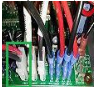
c. Feed Motor Wire (shown in Green)
