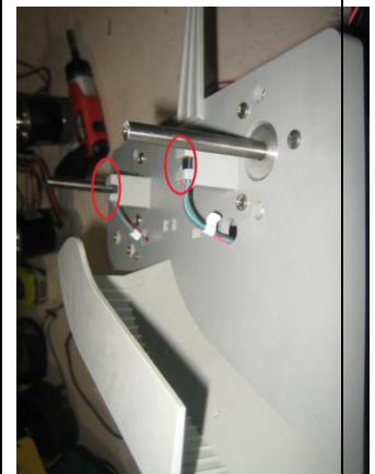
Top and Bottom Server Motor Snap-in Sensor Wires (marked in red)
