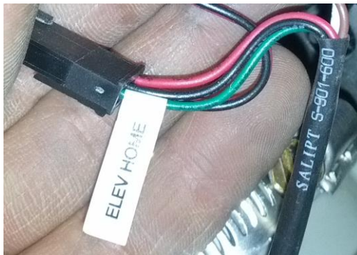
Diagram C.) Elevation Home wire (red, black, and green).
