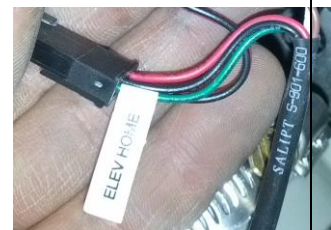
Diagram C.) Elevation Home connection red, black, and green.
