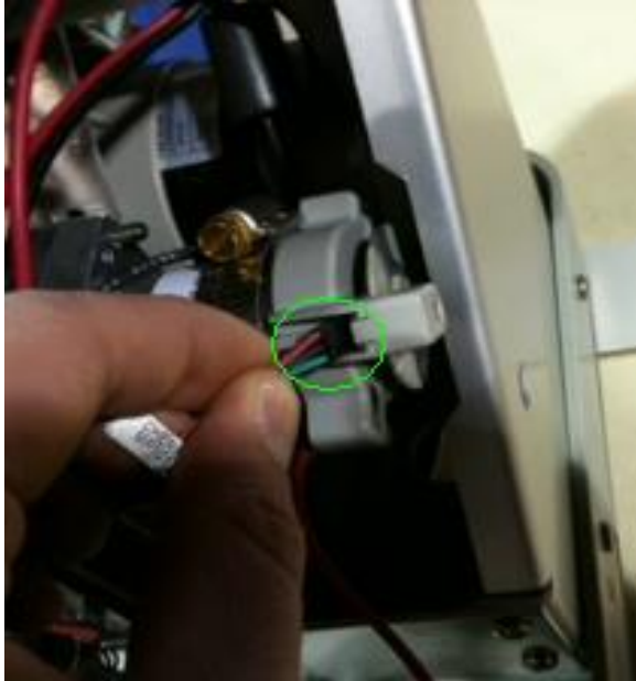
Elevation Motor (Snap-in Sensor highlighted by green circle.)
