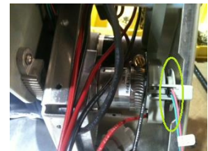
Elevation Motor (Timing Disc highlighted in green). Visible through the rear Circuit board side of the hopper
