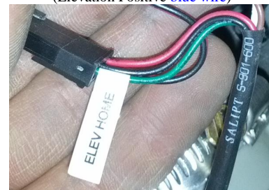
Diagram B.) Elevation Home connection red, black, and green.
