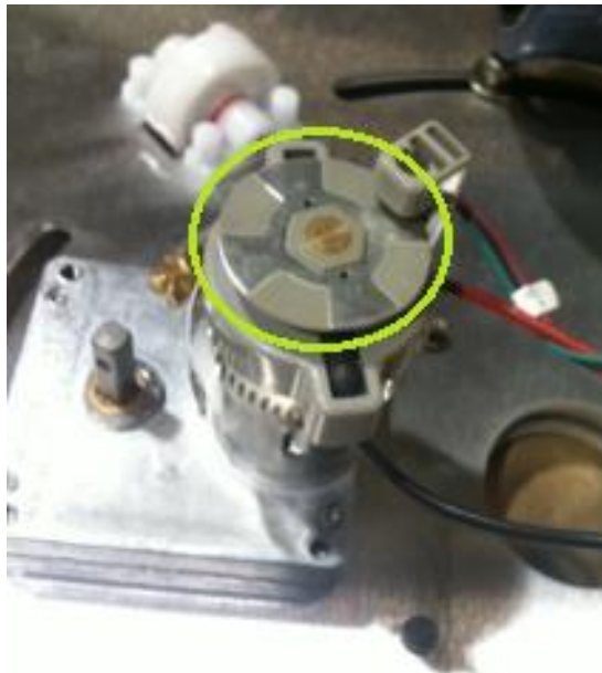
Sweep Motor (Timing Disc highlighted in green).
