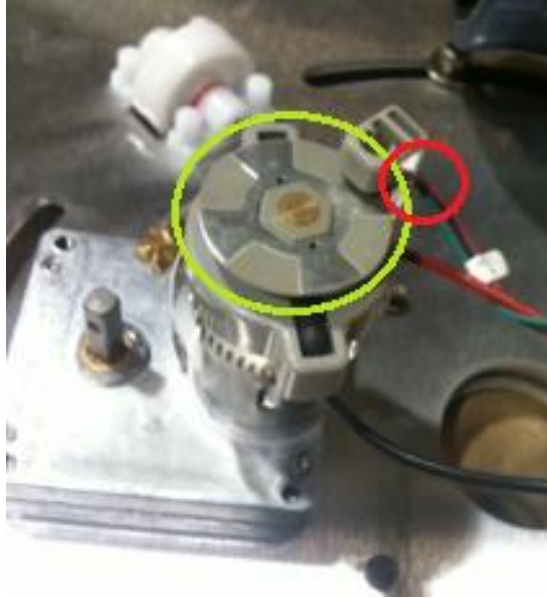
Snap in sensor on Sweep Motor (marked in Red).
