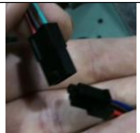
(Vein Harness wires unplugged.)
