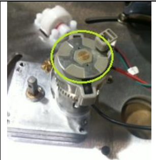
Sweep Motor (Timing Disc highlighted in green).
