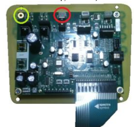
Ground wire location. (Green) Feed Motor location. (Red)
