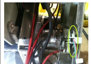
Elevation Motor (Timing Disc highlighted in green).
