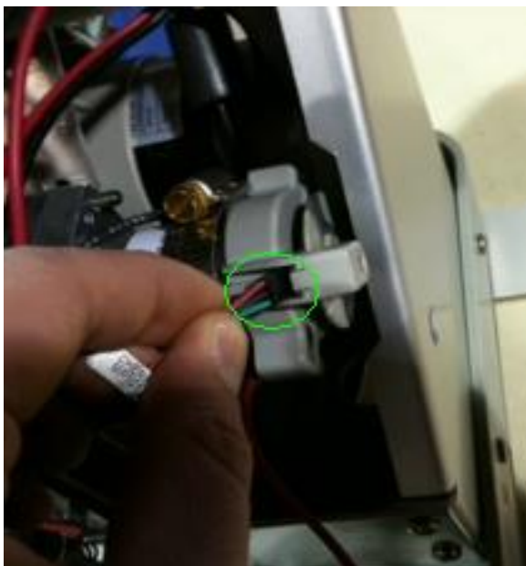
Elevation Motor (Snap-in Sensor highlighted by green)
