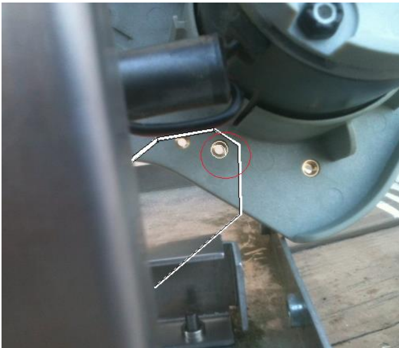
(Elite model 2&3 and Pickle 2, link, shoulder bolt, location).
