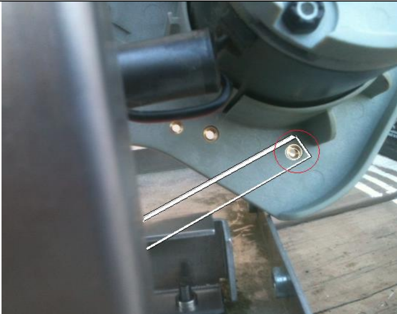
(Elite model 1 link, shoulder bolt, location)
