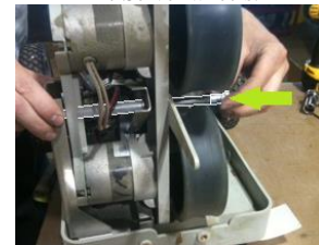
The Yoke Bolt being installed.
