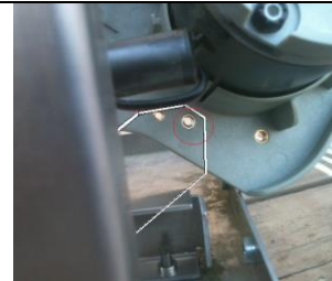
Elite 2&3 and Pickle 2 link and shoulder bolt.
