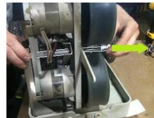
The Yoke Bolt being removed.
