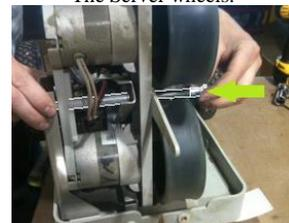
The Yoke Bolt being installed.
