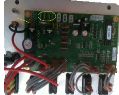
The Green Line shows Battery Negative Tabs, the Green Circle shows the Server Motor Wire location.
