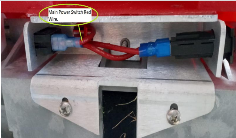
Main Power Switch Red wire (underneath the rear of machine).
