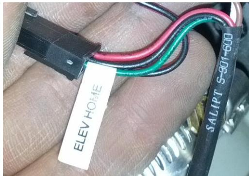
4. Unscrew the control panel, and check the Vien Sensor Harness connection (marked as J10) on the circuit board. Disconnect this by pinching on the two longer sides, and pulling up. Blow it out and then reconnect it.
