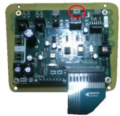
Control Panel J14 Elevation plug.
