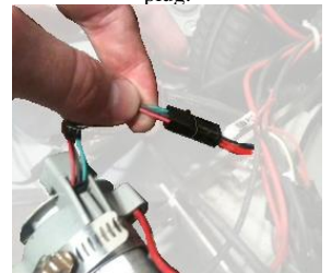
Elevation Quick disconnect location.
