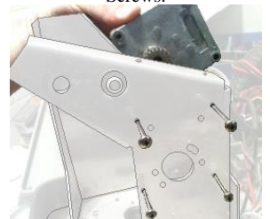
Removing Elevation motor.
