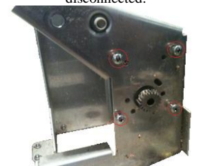
Unscrewing Elevation Motor Screws.
