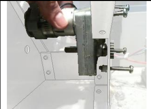
The Elevation Motor being held into place.
