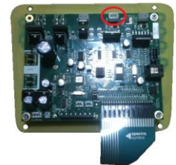
Control Panel J14 Elevation plug.
