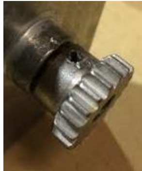
Spring Pin and Spur gear flush.
