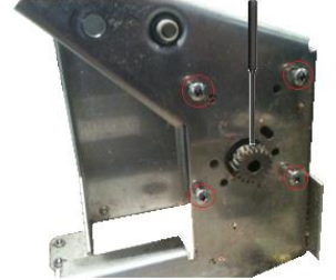
Hammering spring pin into Spur Gear and Motor Shaft.
