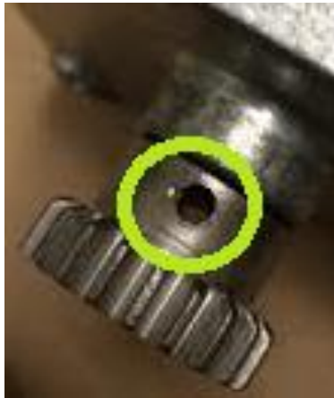
Spring Pin Hole on Spur Gear and Motor Shaft.
