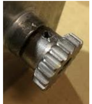
Spring Pin and Spur gear flush.
