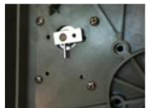
Sweep Link in place with Spring Pin (Hammer up until flush)
