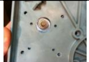
Sweep Motor being removed (screws removed)
