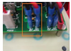
b. Bottom Server Motor (marked in Orange).
