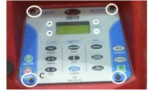
4 Control Panel Screw Locations.
