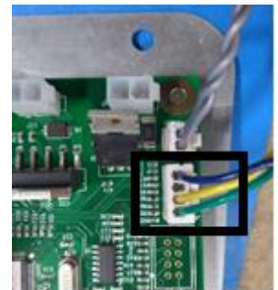
n. 2-Line Wires (marked in black)
