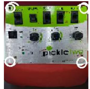
4 Control Panel Screw locations.
