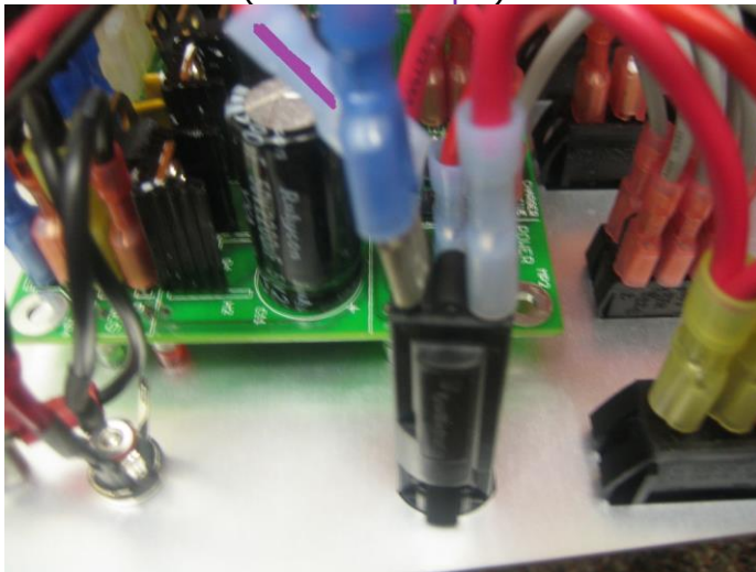
j. XLR Charger Jack red (positive) wire to the prong on the reset switch. (Marked in Purple)
