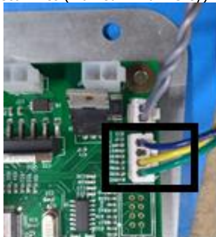
n. 2-Line Wires (Marked in Black).
