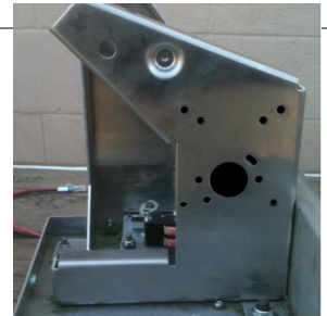
Davit Center with Elevation Motor removed.
