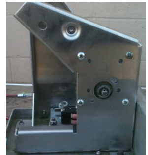
Davit Center with New Elevation motor installed.
