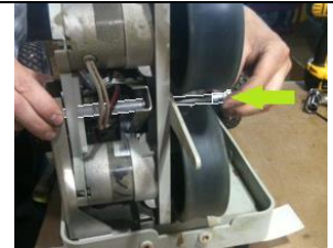
The Yoke Bolt being removed.
