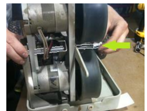
Yoke being fasten to Davit Assembly by Yoke Bolt..
