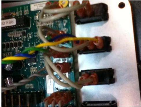
Yellow Blue, and Green Wires (2-line wires) 2 grey wires (ball detection wires).
