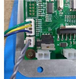
White clip with Green, Yellow and Blue for the 2-line on the elite 3.10 and Pickle 2.10. white clip with 2 grey wires for the ball detect switch (located underneath the 2-line clip).
