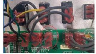
Ball Detect Switch (Ball SW) on Pickle 2.
