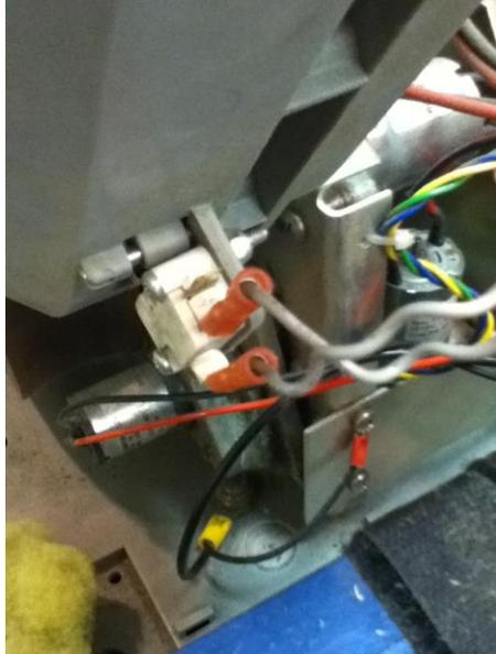
Ball Detection Switch (Elite 3, 3.10, and Pickle 2) with grey wires connected.
