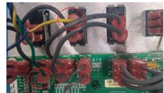
2-line location yellow and green only (blue wire is not connected) on circuit board for Pickle 2.
