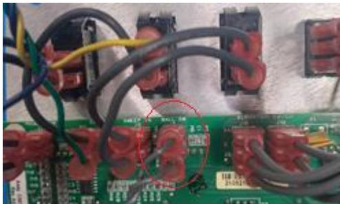
Ball Detect Switch (Ball SW) on Pickle 2.
