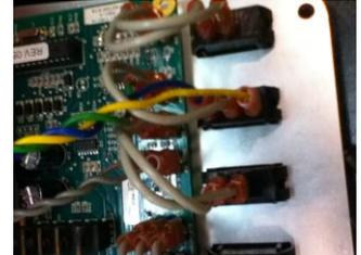
Yellow Blue, and Green Wires (2-line wires) 2 grey wires (ball detection wires) (Elite 3 and Pickle 2).
