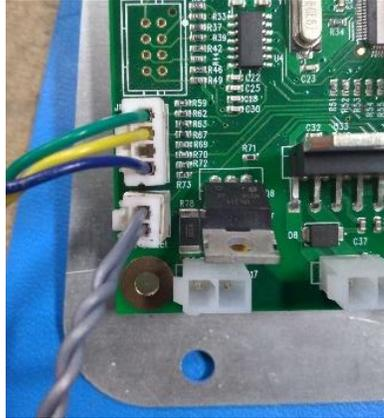
White clip with Green, Yellow and Blue for the 2-line on the elite 3.10 and Pickle 2.10. white clip with 2 grey wires for the ball detect switch (located underneath the 2-line clip).
