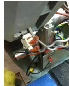
Ball Detection Switch with grey wires connected (Elite 3, 3.10 and Pickle 2)
