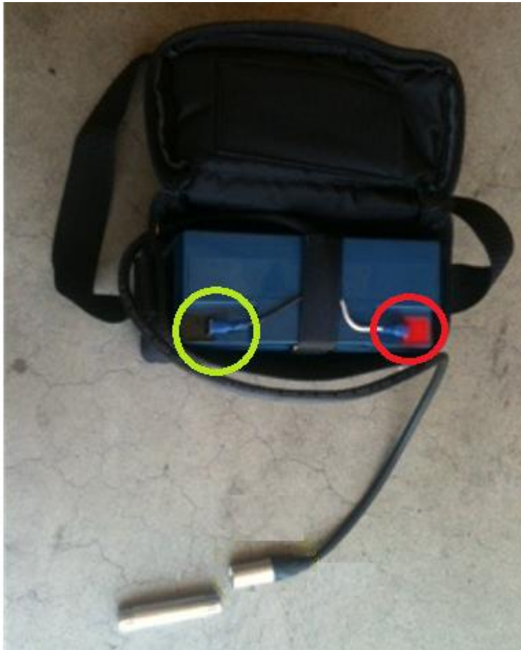
Battery Positive wire (white wire) marked in red. Battery Negative Wire (black wire) marked in Green.
