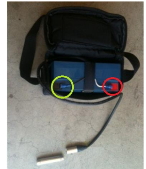
Battery Pos (white wire) marked in Red, battery negative (black wire) marked in Green.
