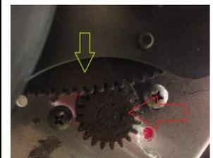
Arc Gear marked in Green. Spur Gear marked in Red.
