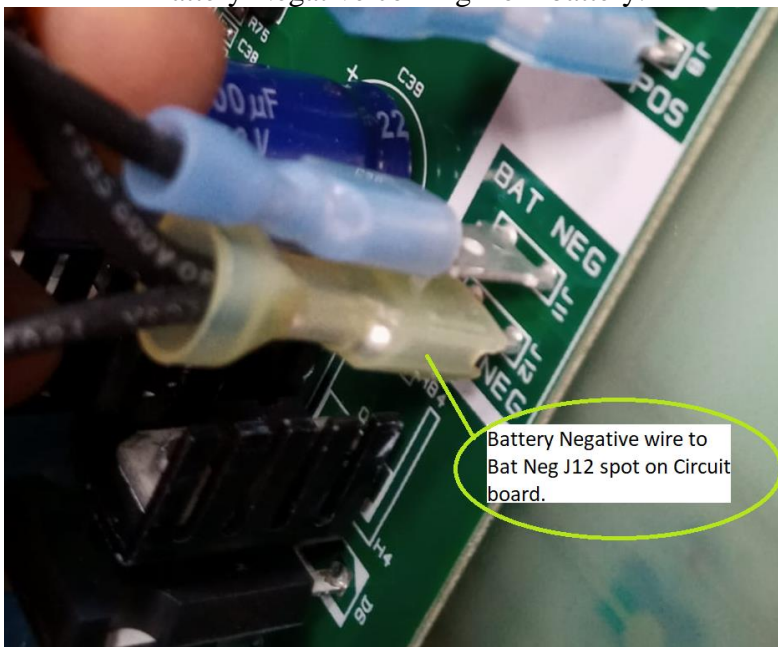
Battery negative connected to Bat Neg J12 on circuit board.
