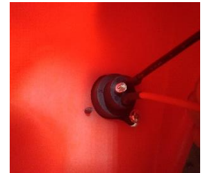
XLR wires inside of red case (where the wires come from the XLR charging port).
