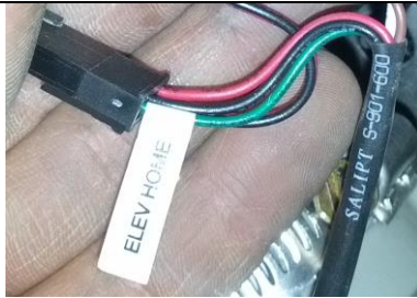
Diagram D.) Elevation Home connection red, black, and green.
