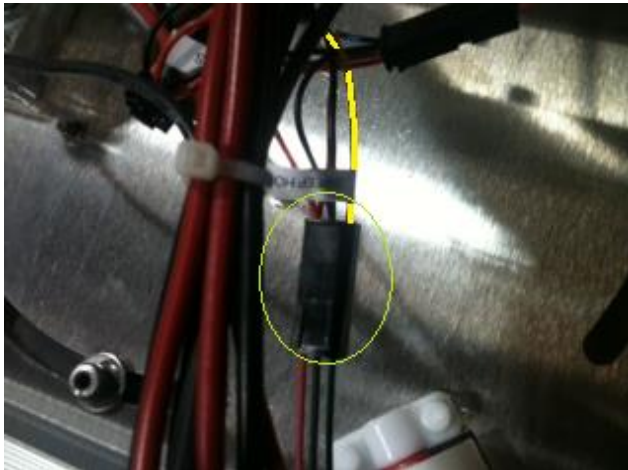
Sweep Home quick disconnect (red, black, and yellow wires).
