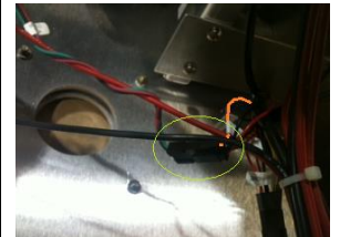
Sweep Pos quick disconnect (Red black and Orange).
