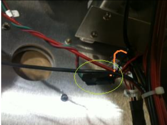
Sweep Pos quick disconnect (Red black and Orange ).
