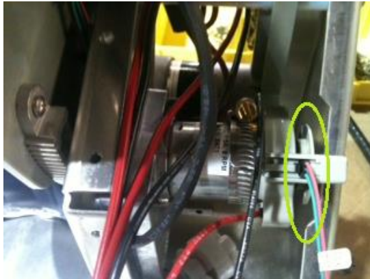
Elevation Motor (Timing Disc highlighted in green).
