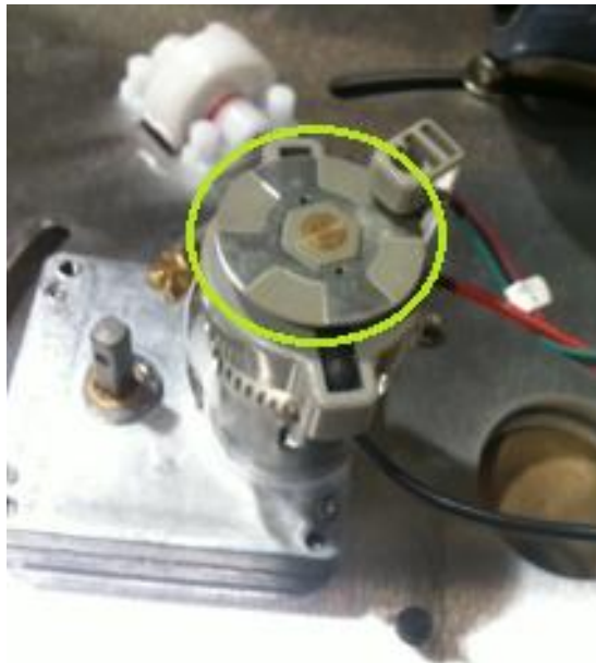
Sweep Motor (Timing Disc highlighted in green).
