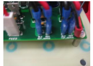
Server Motor Connections
