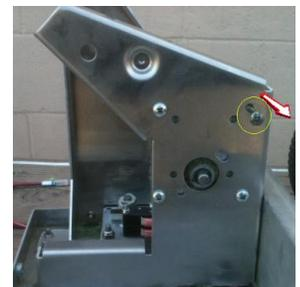
Remove Elevation Motor Screws.
