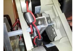
Slide yoke bolt throughlong plastic spacer and davit
