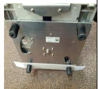
Rubber feet installed on platform.
