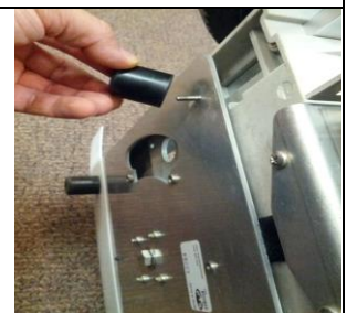
Foot being fastened to platform.
